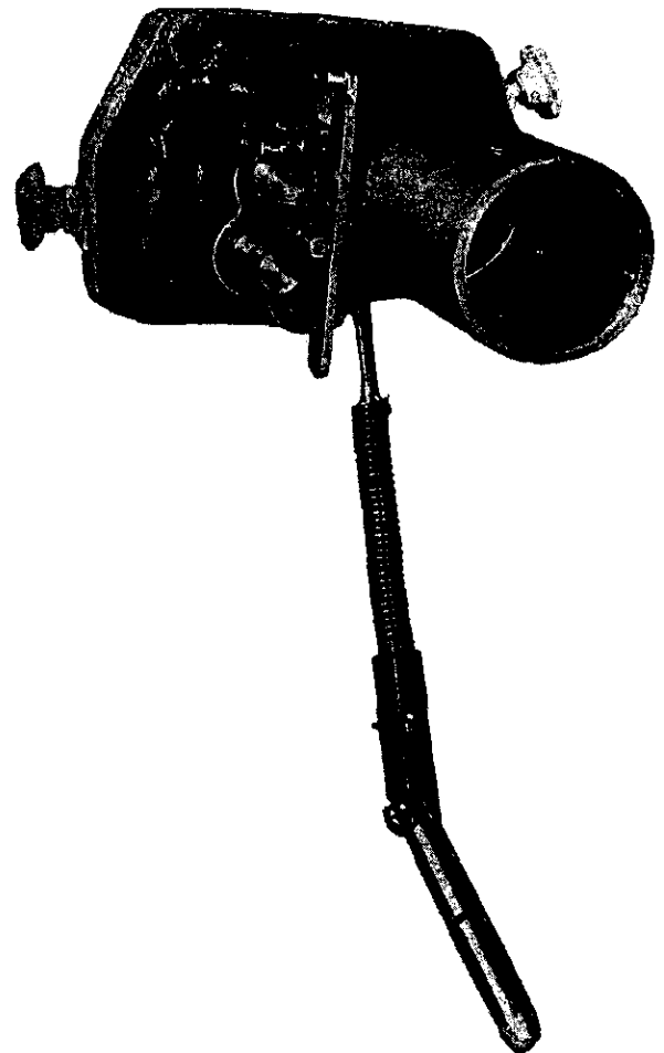
Fig. 142—Control valve assembly and draft plunger linkage after removal from hydraulic lift housing.
